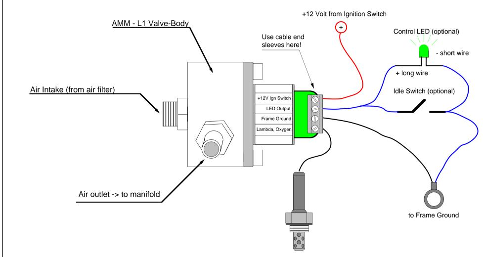
1-wire Oxygen Sensor mounted to exhaust near Cyl. outlet
