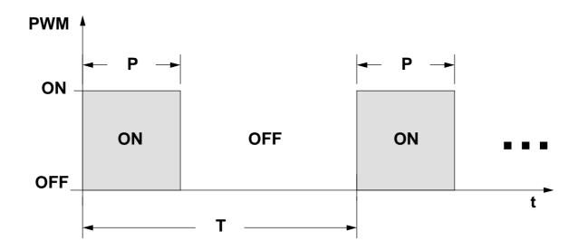
Peak-Current-Limit relates to real-time current during the active PWM-pulse ON-time (P).
