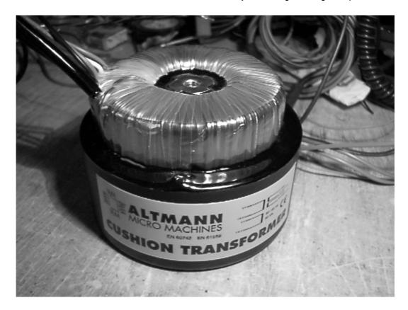
The "Altmann Cushion Transformer" is mounted to the aluminium profile of the power supply housing by a central screw, while it "sits" in a polyurethane cushion. This construction ensures absolute silence.
