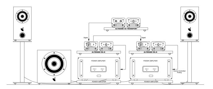
Two ALTMANN DA-R units are connected in a daisy chain to one digital output device (f.e. ALTMANN CD-TRANSPORT).
