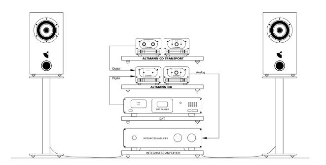
The ALTMANN DA drives an integrated amplifier (top) or a preamp / poweramp combination (bottom).
