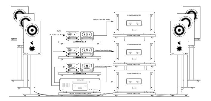
Three ALTMANN DA-R units are connected to a multichannel digital input device, that delivers 3 stereo pairs of digital pcm output data.
