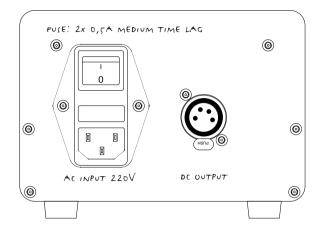
Please check that the voltage rating under the AC input socket (220V in this case) matches your AC wall outlet.
