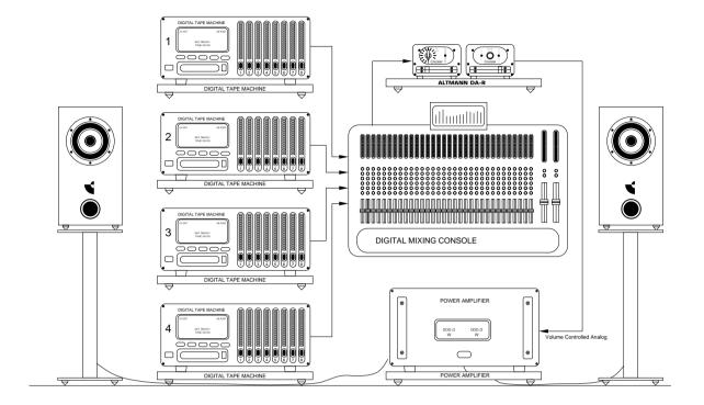
Four digital 8 track tape machines are connected to a 32 track digital mixing console.
