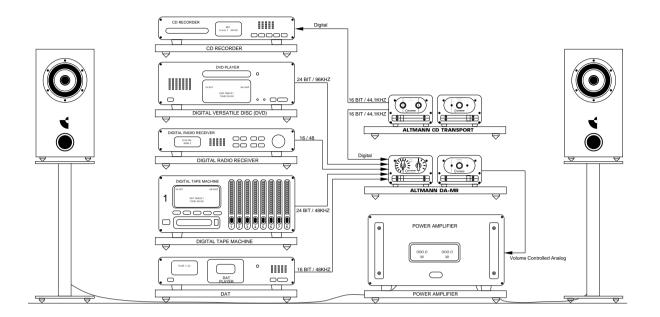
The ALTMANN DA-MR is connected to several digital input devices, that can be selected on the frontpanel.
