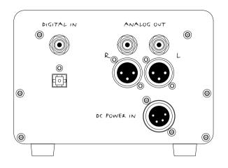
Each ALTMANN DA converter system has a stereo pair of Cinch and XLR analog outputs.
